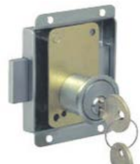
latch #3273Z; 25 mm backset, brass chrome plated; also with 20, 30 mm backset For door thickness from 5/8" to 1 3/16."
